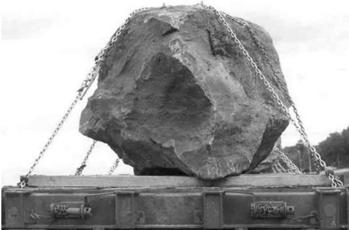
*Chain is used to secure large boulders*
