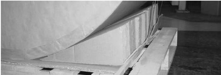
The method used to prevent rolling must not become unfastened or loose while the vehicle is in transit.
