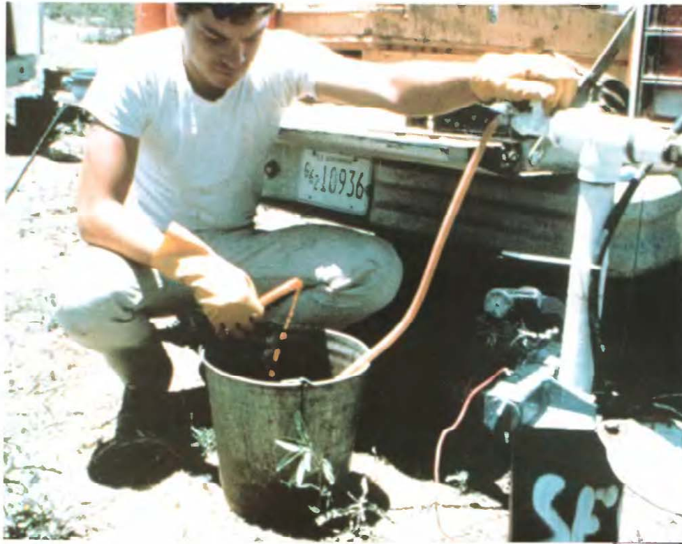
Sampling acidic, metal-laden ground water from monitoring wells near Globe, Arizona. For at least the past 40 years, acidic water originating from mining and milling process solutions has caused extensive ground-water contamination in this copper-mining area of Arizona. In 1986, water from several wells in the area contained concentrations of aluminum, copper, and iron exceeding 100 milligrams per liter. (Photograph by James H. Eychaner, U.S. Geological Survey.)
