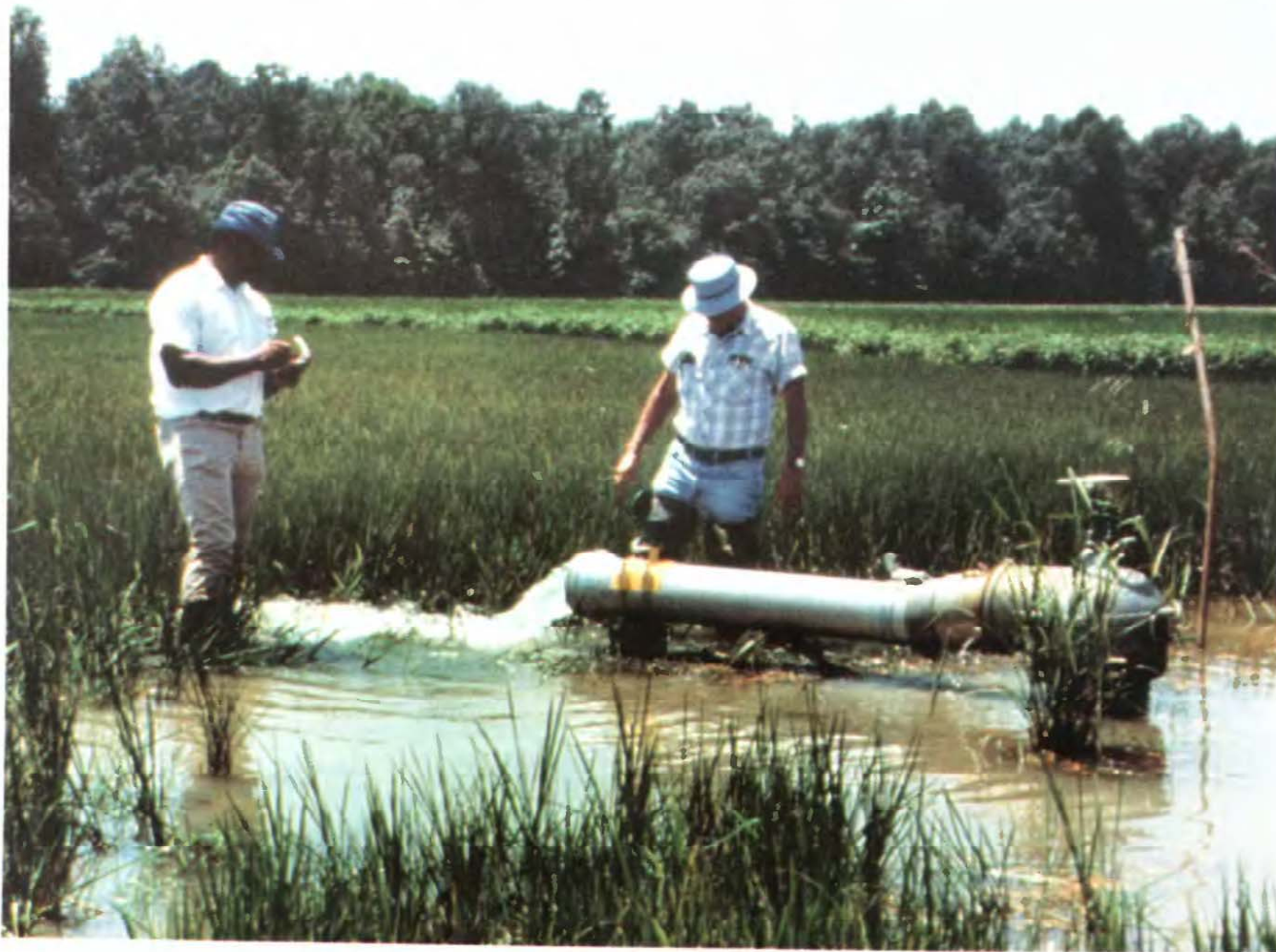
Measurement of water flowing from an irrigation well in a rice field. The U.S. Geological Survey in cooperation with the Arkansas Geologic Commission collected well yield and water-quality information from the alluvial aquifer near Brinkley, Arkansas. The results of chloride analyses were used to map the extent and magnitude of saltwater intrusion into the alluvial aquifer. (Photo courtesy of the U.S. Department of Agriculture, Soil Conservation Service.)
