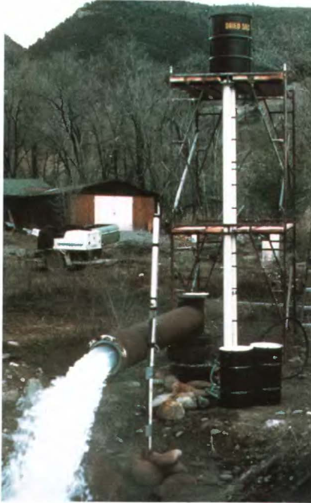
Aquifer testing in the Redstone 21-9 geothermal well at Glenwood Springs, Colo., November 1984. Tera Therna Inc. participated with the U.S. Geological Survey, Wright Water Engineers, and the U.S. Bureau of Reclamation in conducting the test. The test was conducted to analyze the hydraulic properties of the Leadville Limestone and the Dyer Dolomite, to determine the degree of interconnection between these aquifers and the overlying alluvium, and to determine the effects of discharge of water through the wells on the nearby springs. During the 4-day test, the discharge of the well decreased from 2,300 to 1,740 gallons per minute and the temperature of the water ranged from 45 to 49° C. (Photograph by Arthur Geldon, U.S. Geological Survey.)
