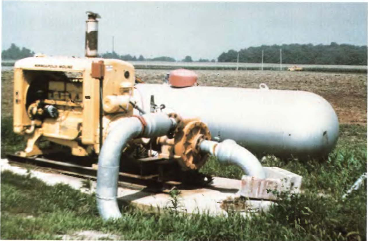
Natural gas powered centrifugal pump used to irrigate crops in Mason County, Illinois. The County has extensive pumpage for irrigation from the shallow sand and gravel aquifer in the area. (Photograph by Walter Lembke, Department of Agricultural Engineering Sciences, University of Illinois.)
