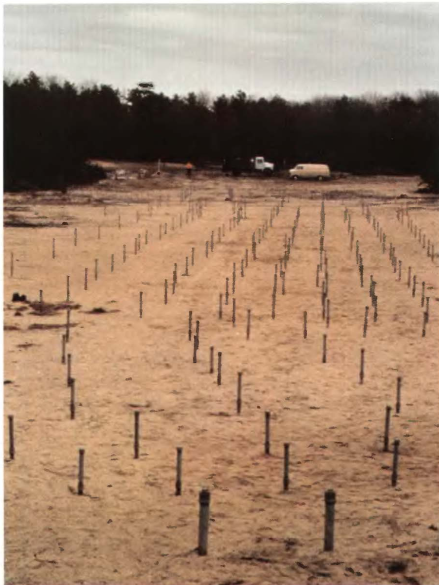
Multilevel observation wells at US Geological Survey study site, Cape Cod, Massachusetts. Research on contaminant transport and dispersion in an aquifer is being conducted using this array of 640 observation wells. Water samples can be obtained from 15 different depths in each of the wells. (Photograph by Denis R. LeBlanc, U.S. Geological Survey.)
