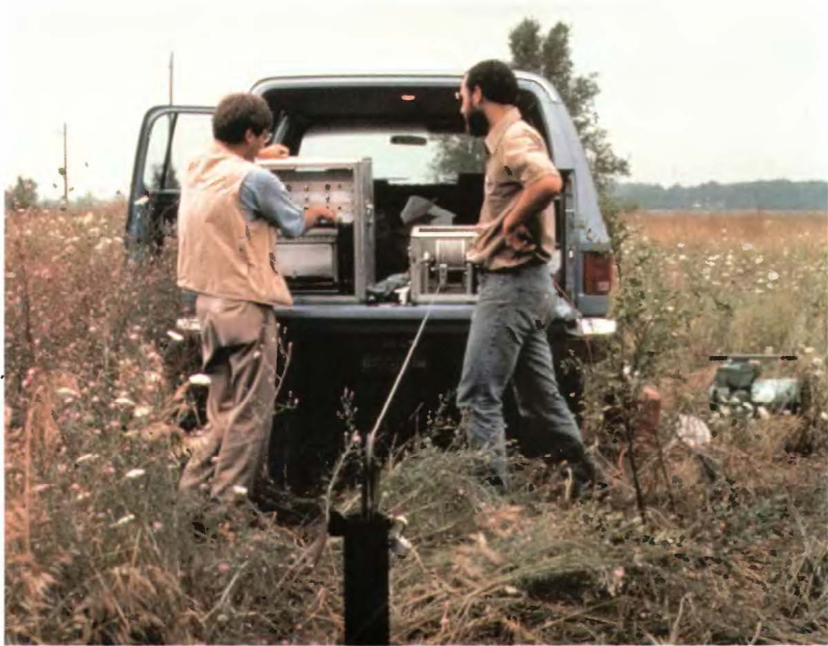
Geophysical well logging being conducted by U.S. Geological Survey personnel in southeastern Michigan. Information about the thickness, lithology, and properties of the strata penetrated by a well can be obtained using a variety of geophysical well-logging probes. (Photograph by Steve Rheaume, U.S. Geological Survey.)
