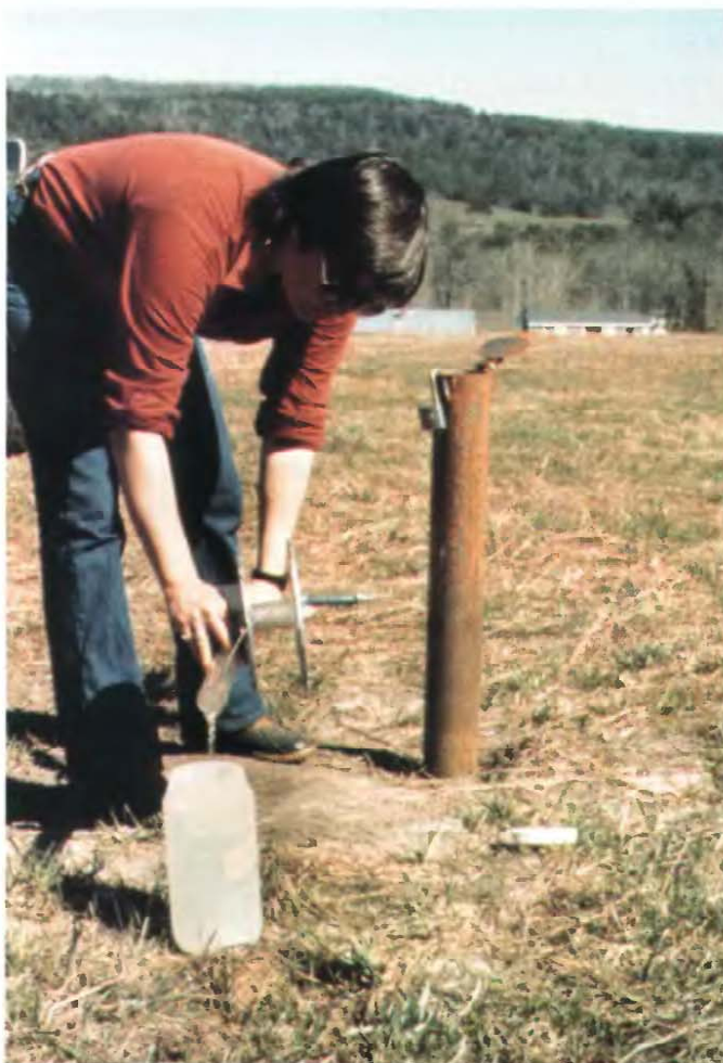
Vermont Department of Environmental Conservation employee Marsh Thompson obtains a water sample for chemical analysis from a monitoring well in Windsor County, Vermont, as part of an investigation of septic systems as sources of nitrogen in ground water. (Photograph by James W. Ashley, Vermont Department of Environmental Conservation.)
